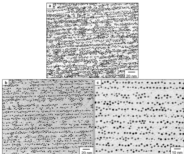
Figure 3. TEM images of 3.4 nm DT–Au nanoparticles on ridge-and-valley carbon layers. (a) Prepared by a drop method. (b) Prepared by a dip method. (c) A magnified image of (b).
